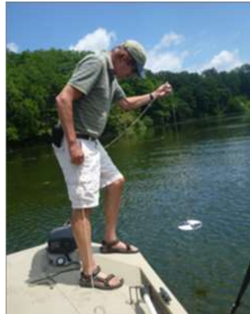
Figure 3. Checking water clarity with Secchi disk.
